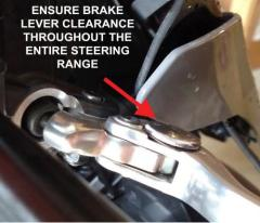
sure that the throttle cables are not encumbered through the entire range of motion and make sure that your throttle closes properly throughout the ENTIRE range of motion before attempting to ride the motorcycle.
